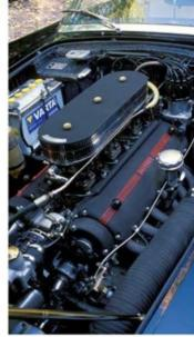
The engine in the 250 GT Capriclet Series Iwas a Colombodesigned sintydegree V12 with a bcrexstrokeof73 x 68.8 millmeters (2870 x 2.316 inches) displacing 2.953 cubic centimeters (180) cubic inches). The valve-operation was by a single-overhead camehaft on each bank with roller followers and rocker arms to inclined valves. With three twin-choke Weber carburetors and a compression ratio of 8.51, output from this engine was 240 horsepower at 7.000 revolutions per minute.
