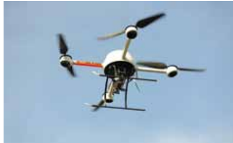
Above: A German police drone from 2012, equipped with camera surveillance for aerial filming and monitoring.
