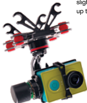
Left: The cheaply-priced XiaoMi Yi 3-axis brushless BL Gimbal works with most quadcopters.
